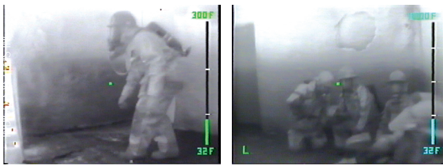
By imaging in high gain (left) and low gain (right) states, the camera reduces dynamic gain demands on the FPA.
