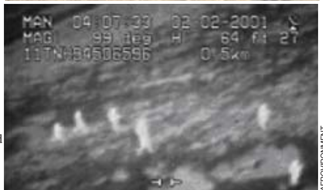
FIGURE 2. The Pointer unmanned aerial vehicle (top, at launch) uses a thermal IR camera for surveillance. An IR image from a UAV flying at 65 ft above the ground shows personnel (bottom).
