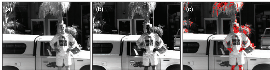
Fig. 4. Image from an InGaAs camera with a 900–1000 nm filter (a) and a 1400–1600 nm filter (b). The third image (c) shows the difference between the other two images, false-colored in red and overlaid onto (a). Exposed skin and vegetation are clearly apparent.
