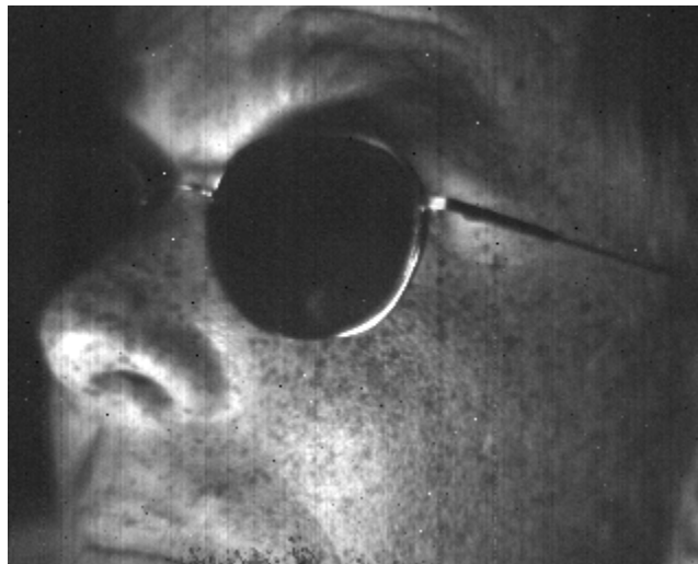
Figure 5: A face illuminated with a uv light, imaged by ENG 1. Dark skin blotches are sun damage revealed by uv illumination. 5
