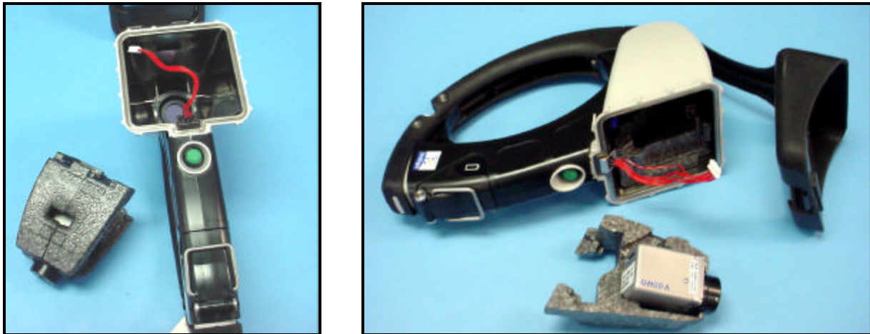
Figure 8: Omega™ removed from E5000 housing (enclosed in foam shell)
